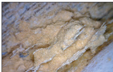
Anobiid powderpost beetle and damage
