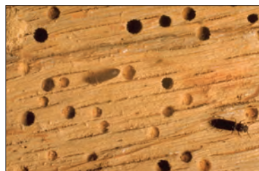
Lyctid powderpost beetle and damage (below)
